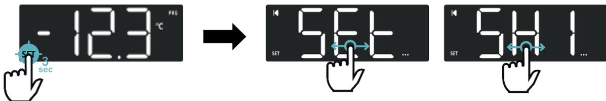
From the Programming Menu it is possible to access the Setpoint Menu by holding down the SET icon for 3 seconds. The SET and PRG function icons flash until the Setpoint menu is unlocked. The Set label indicates that the temperature set point is unlocked. Use the horizontal swipe to move within the Setpoint Menu between temperature and humidity. Press the BACK icon to exit and return to the Programming Menu
